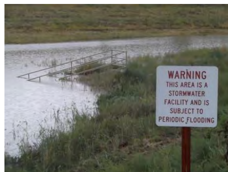
Regional Ponds in the Cottonwood Creek, Dove Creek, and Windmill Creek basins detain storm flows and release at a slow rate to keep the runoff peaks from damaging structures
