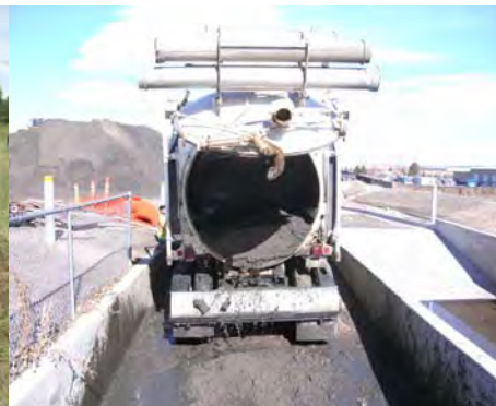
Pipe/Vault Cleaning and Sediment Disposal
